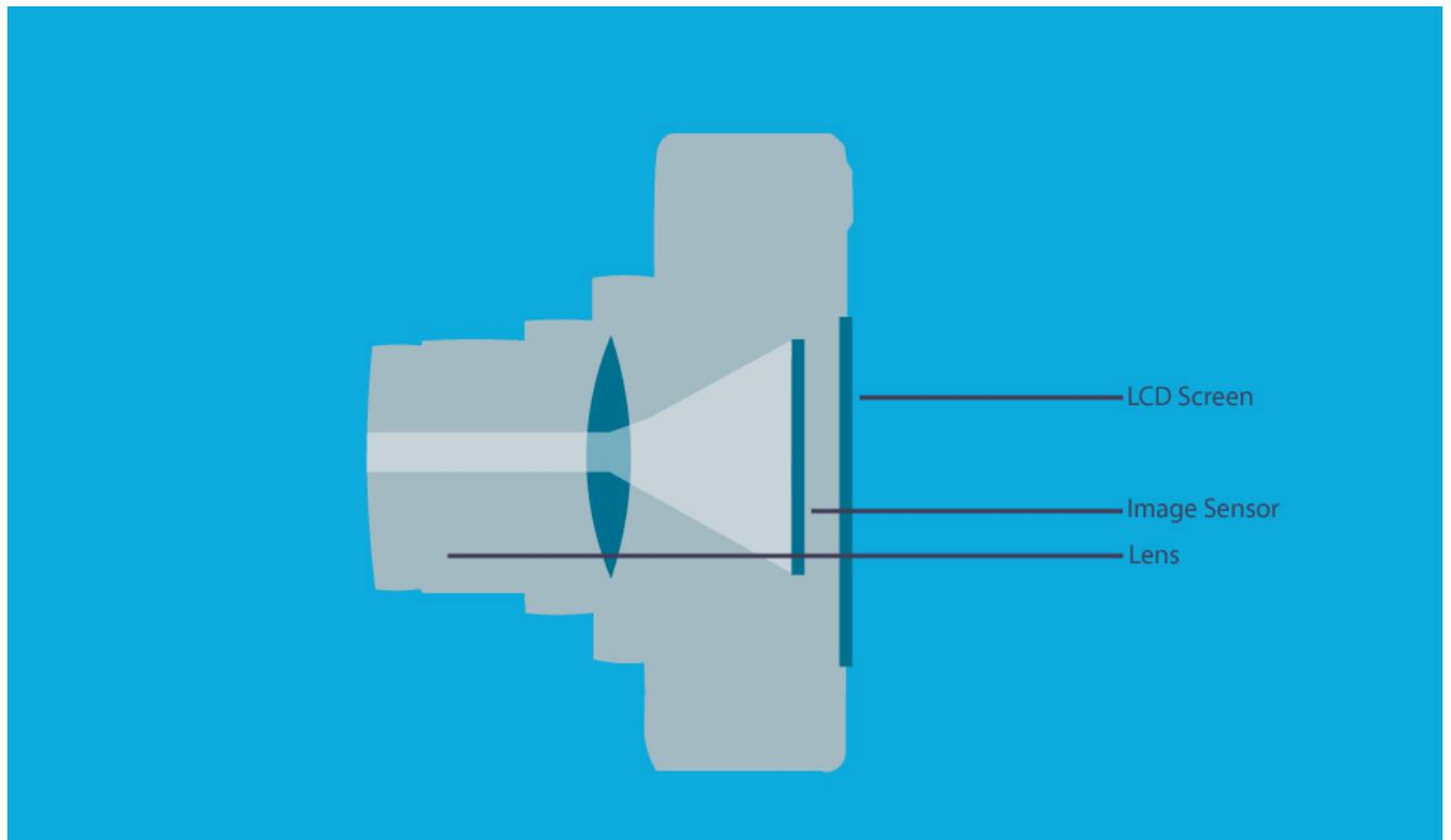
*The basic components of a typical point-and-shoot camera*
