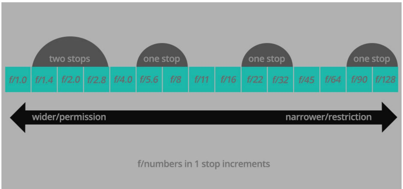
The smaller the number, the wider the opening. Therefore, a lens with a larger-diameter barrel and optics will allow a larger opening represented by a smaller *f/stop*. Your lens/camera might allow you to "dial up" different numbers than what is shown above; older manual lenses usually "click" at 1/2 stop increments. These numbers, seen on a digital display, like *f/3.3* for instance, represent 1/2-stop or 1/3-stop ratios.
