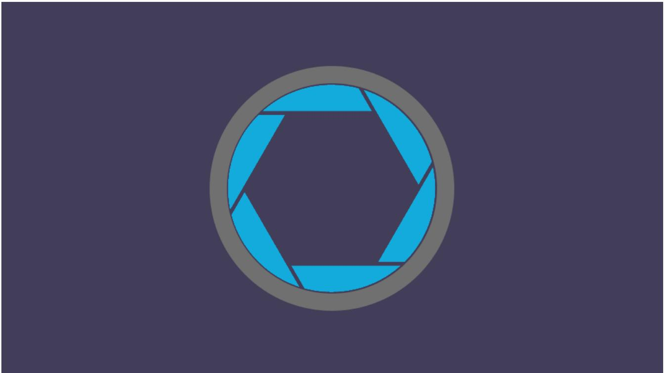
*Aperture is created by a set of blades inside the lens.*
