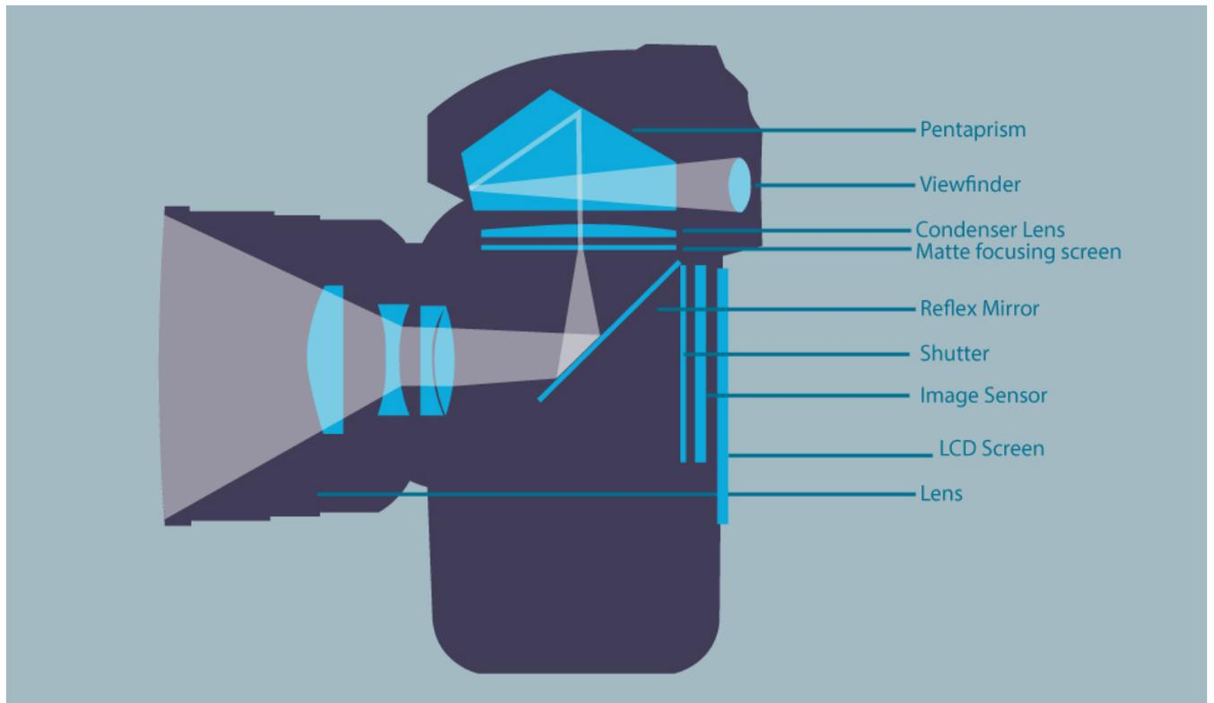
*The basic components of the DSLR*
