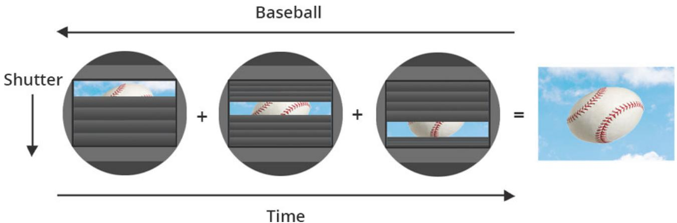
Like most things, the shutter has gone digital. Many modern digital cameras operate an *electronic shutter* that simply powers the digital sensor on for a selected amount of time. Because there is no mechanical function, electronic shutter speeds can be extremely fast. A *global shutter* turns the entire sensor on and off at once, while a *rolling shutter* activates one row of pixels at a time across its width.
